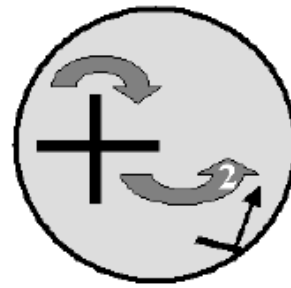
e. Planetary motion (Pan fixed/scrapper moving. The shaft is also rotating following Arrow 2.)
